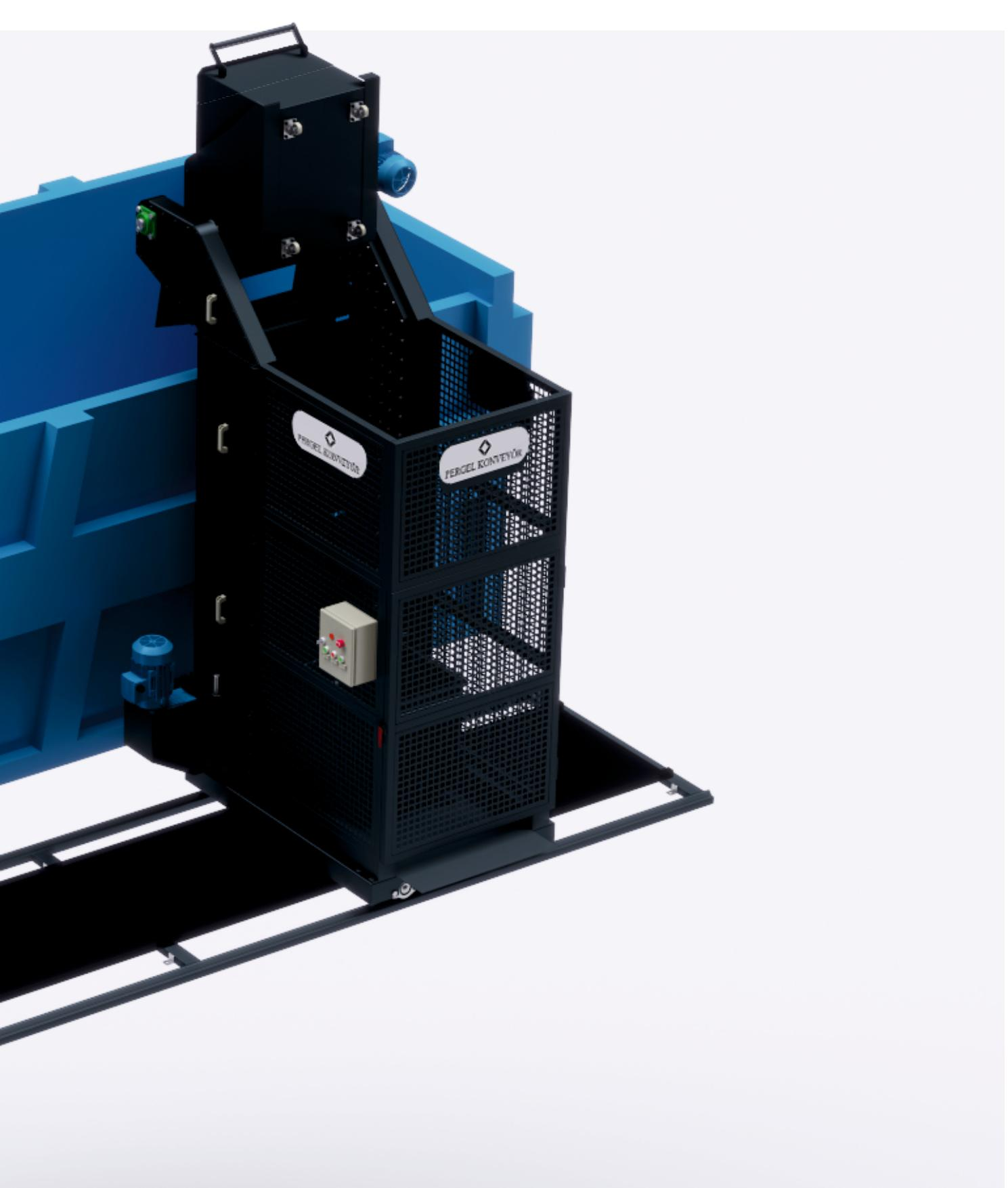
It is used for unloading / loading the chips accumulated from the machine tools to the chip trolley into the conveyor, container or silo at a certain height.
