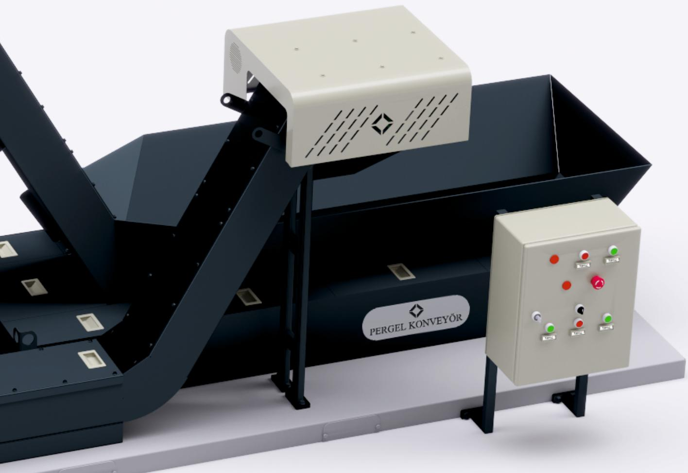
These are complex systems used for the separation of sawdust and cooling/cutting fluid mixture after machining in machining. In the system, steel pallet chip conveyor, bottom scraping conveyor, vibro-sieve and centrifuge are used in coordination. After the cooling/cutting fluid is separated, it is filtered again and pressed back into the system, thus recovery is achieved. The system ensures that the sawdust is dried, making the sawdust more valuable and reusing the recovered oils.
